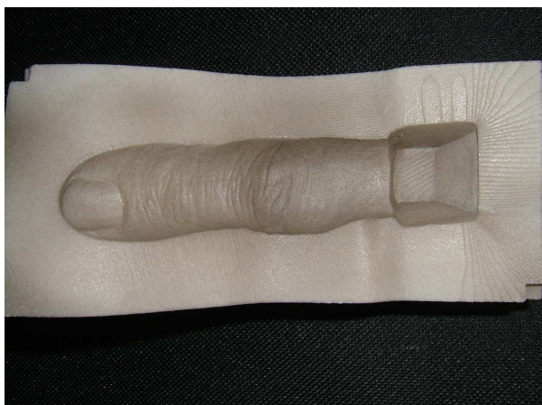
Fig 5: At the last trial, SLS technology was used to produce a tool for manufacturing a silicone finger epithesis
