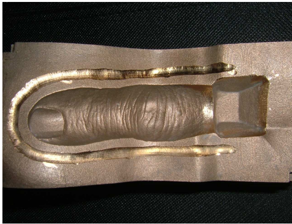
Fig 4: DMLS technology was used to make a mould for manufacturing silicone finger epithesis
